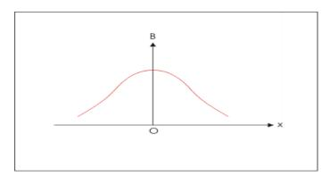
away from the centre on either side of the loop. Variation of B along the axis of a circular current loop
