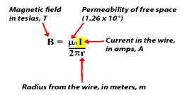
The equation gives us the magnitude of the magnetic field and direction by right hand grip rule.
